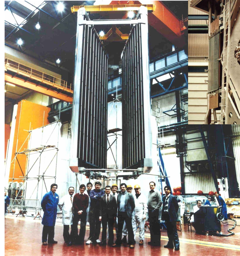
JET NB Injector cryopump
